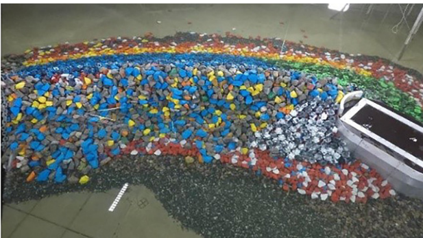
Figure 12. Rear-side damage with 15–22 t rock after overload test
