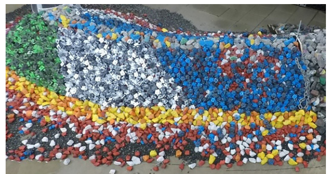
Figure 11. Trunk section with 15 t units after overload conditions
